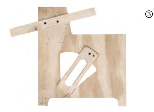
To the left is an Atwood-Hamlin Bracket Jig with upper sticks and bracket angle that will need to be adjusted. Once these are adjusted, by following the instructions below, you will be able to use the jig as a template for each pew keeping the installation process consistent.<sup>3</sup>
