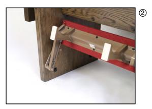
Raise the kneeler up so that the kneeler legs are just inside the top rail. This allows enough room for a person to walk between the pews without hitting their legs. Now, put the other screws in the bracket.<sup>2</sup>
