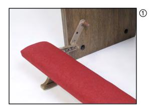
Set up the first Atwood-Hamlin Kneeler in a position comfortable for kneeling (preferably 8" out from top rail of pew). For now, just mount the center screw into the Atwood-Hamlin Bracket at approximately a 45° angle to hold the bracket in place until the final adjustments are made. ①
