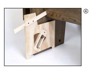
Set up the bracket jig over the bracket you have just attached to the pew. Place upper sticks against the jig allowing an end to butt up against the back of the pew. This shows the distance the bracket is placed from the back of the pew. Set upper sticks with screws. And last, set the angle on the bracket with screws in order to hold its position.<sup>4</sup>
