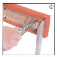
2. First, put the kneeler in the up position. Remove the screws that attach the kneeler pad to the V-shaped metal support bar.
