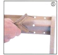
5. Replace with the new leg using the screws provided. (Note the circular tabs on the top of the replacement leg. They should be inserted in the holes on the support bar where the old leg was removed.)
