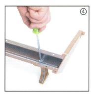
4. Remove the screw that attached the old leg to the support bar and remove the leg.
